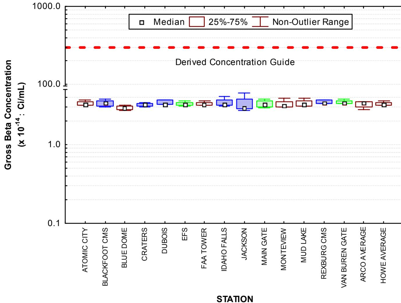
**Figure 9. September gross beta concentrations in air at ESER Program INEEL, Boundary, and Distant locations.** Stations belonging to INEEL, Boundary, or Distant locations are represented by boxes that are patterned with vertical green stripes, no fill, or horizontal blue stripes, respectively. Number of samples (N) = 4 at each location except for ARCO (Q/A-1), Dubois, and Rexburg CMS, where N=3.
