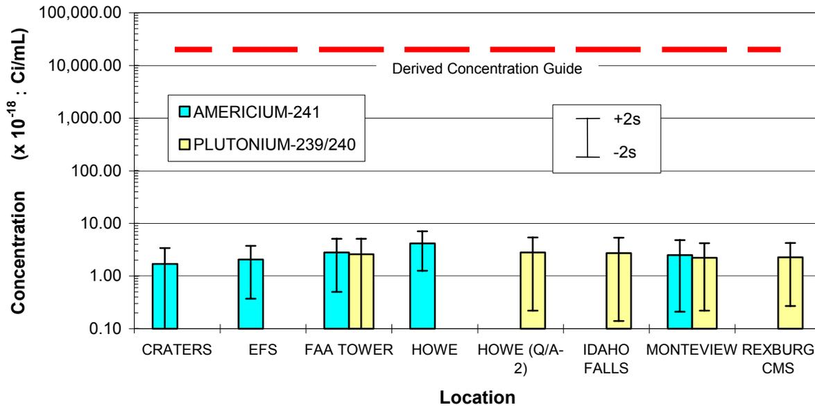
**Figure 10. Specific radionuclides detected in quarterly composite air filters (by locations).**
