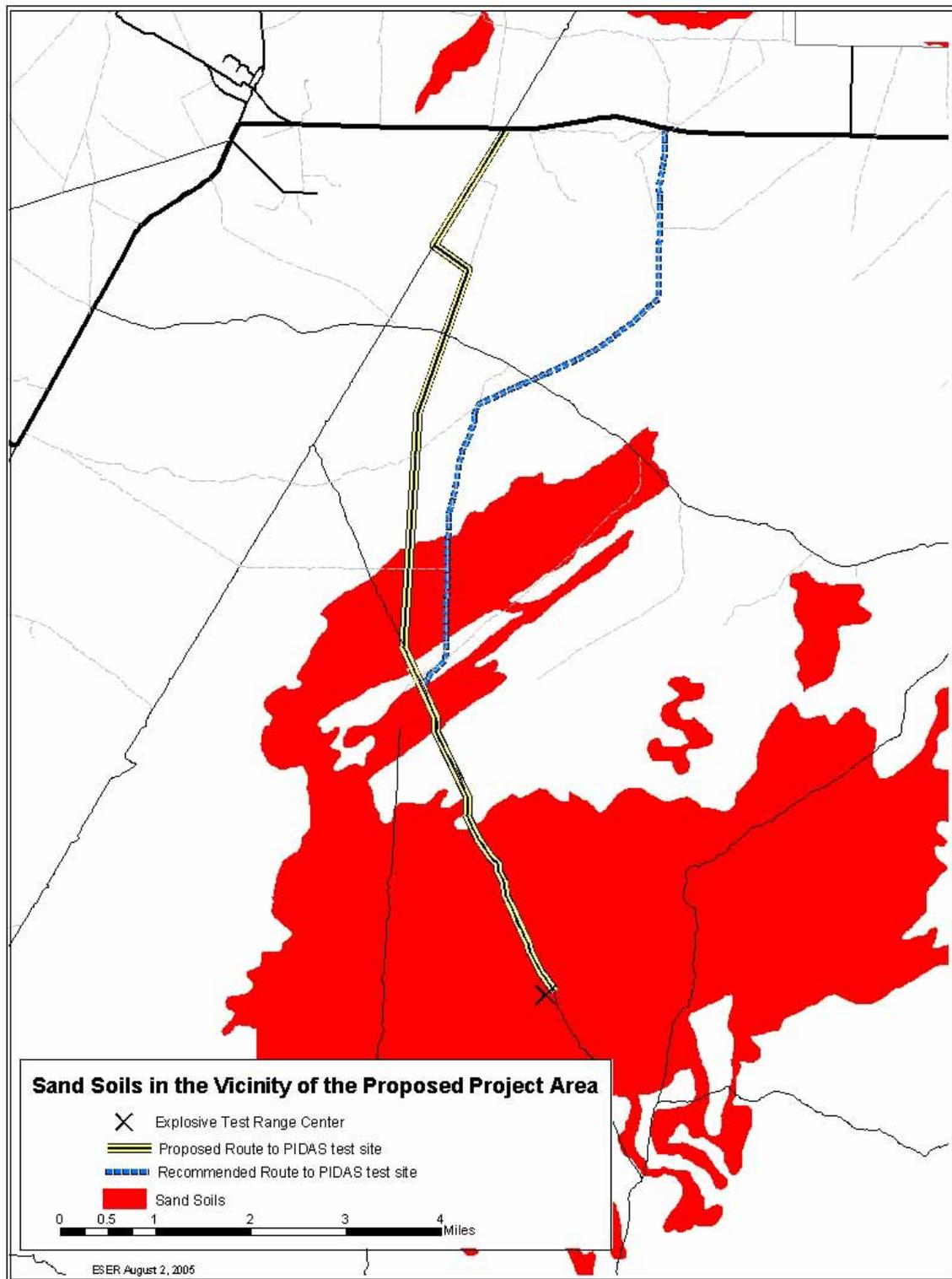
**Figure 4. Soils on and near the proposed test area and the roads to the test area that are at risk to damage from vehicle traffic.**
